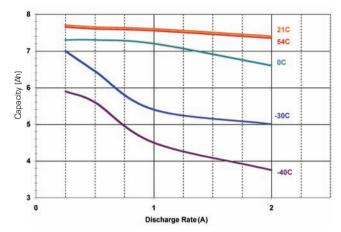
2 A discharge typical curves at various temperatures
